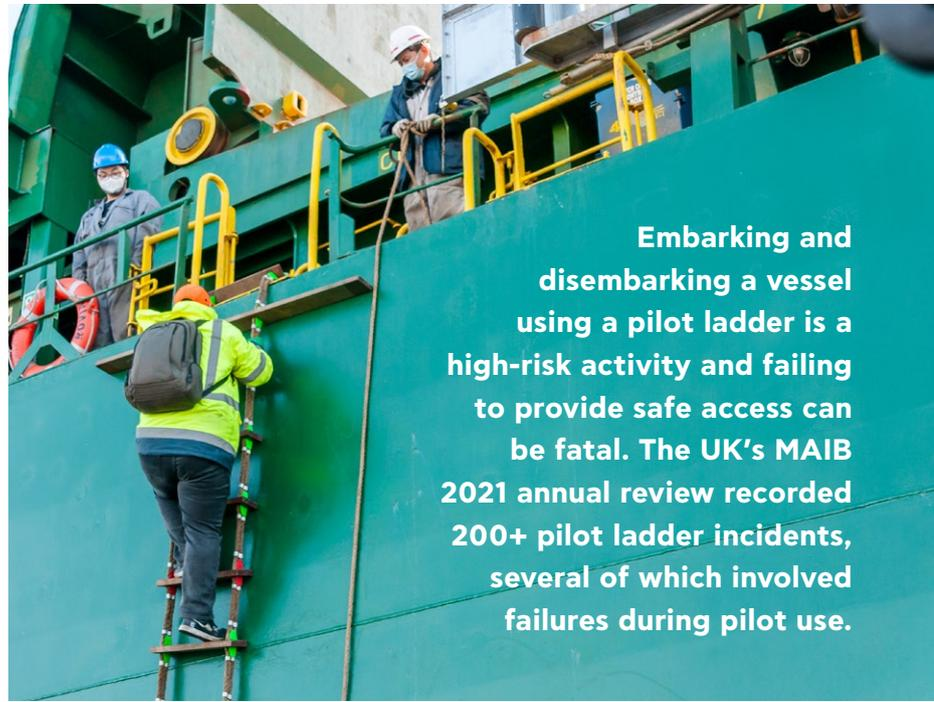
**Embarking and disembarking a vessel using a pilot ladder is a high-risk activity and failing to provide safe access can be fatal. The UK's MAIB 2021 annual review recorded 200+ pilot ladder incidents, several of which involved failures during pilot use.**
